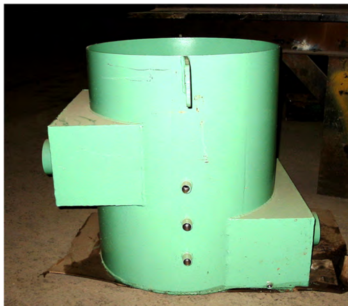
Photograph 1 – Permeameter used in 2007 DE Study
